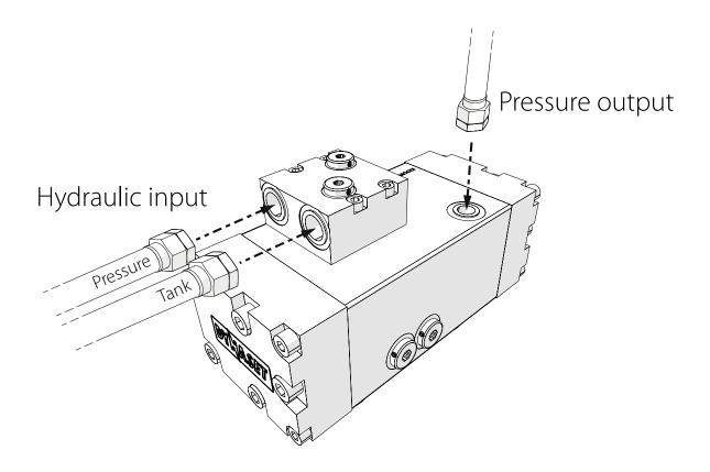
Location of input and output ports may differ between Hydraulic Pressure Insifier models.
