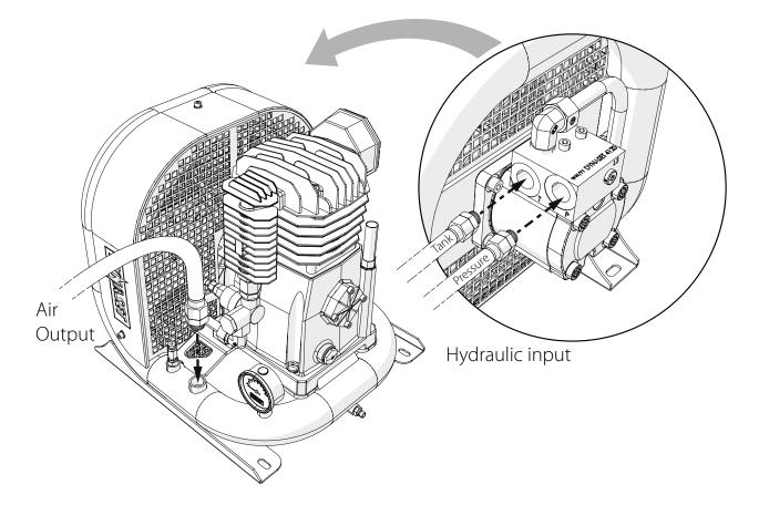
Location of input and output ports differ between Hydraulic Piston Compressor models.
