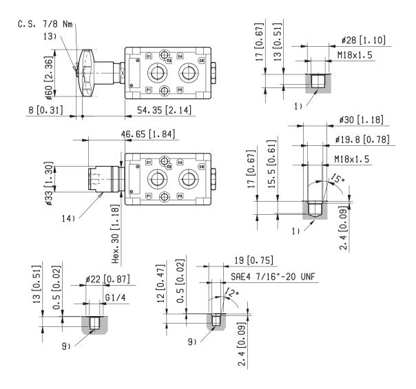
**<sup>13</sup>** Dimensions of optional manual version, push and twist type. Hex 25 mm, torque 22-24 Nm [16.2-17.7 ft-lb].
