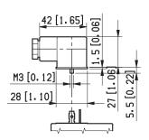
With coils having AMP Junior connector, and with bi-directional diode.
