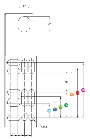
The **BRACKET** realized for **RAAL ITALY** exchangers, sheet metal zinc is unique, and has been studied specifically to be unified on all models.
