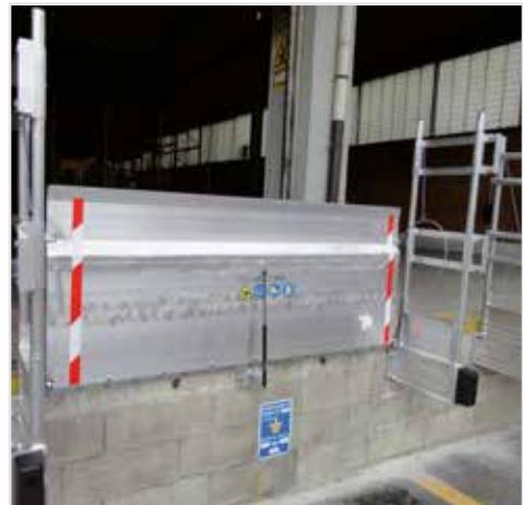
These are platforms for loading and unloading at docks, which can be secured with special steel brackets or pipe connections that can allow the platform to move sideways.
