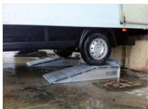
Definitive CLM offers wedges for lifting vehicles that bring the floor of the van up to the level of the loading and unloading docks of logistics warehouses, in order to facilitate and ensure the safety of loading and unloading, and thereby speed up the entire process.
