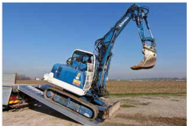
LOAD CAPACITY UP TO 16900 KG | LENGTH FROM 1500 MM TO 5000 MM | EXTERNAL WIDTH FROM 300 MM TO 640 MM
