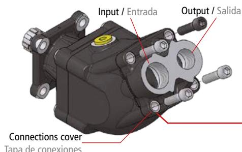
To change the direction of rotation remove the 4 screws and, keeping the distributor body close to the pump, rotate it by 180°
