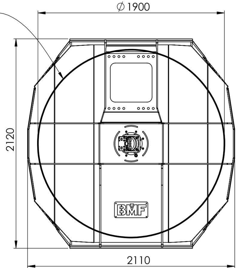
Body is made out of Hardox450
