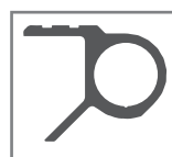
APPOGGIO A TUBO 62mm 62mm TUBE CONNECTION
